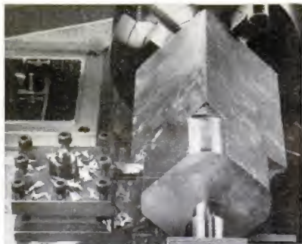
LATHE'S GEARED SPINDLE gives good power for smooth, interrupted cuts as in rounding square stock
